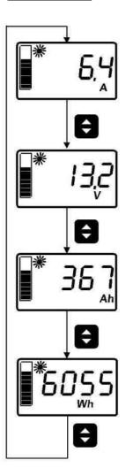
The measuring and display values of the solar installation are scrolled forward via button 1 (left).
