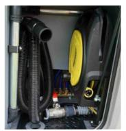
For Mercedes A-class models the fresh water hose drum, the water distributor and the sewage tank drain hose are located together in the central services unit.
