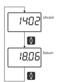
The measuring and display values of the clock and thermometer functions are scrolled forward via button 2 (center).
