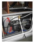
The heating system includes a water heater with the capacity of approx. 8.5 liters of fresh water. It is possible that air can accumulate in the pipes of the water heating. Please use venting screws on the radiators within the seating areas, kitchen and sleeping areas to release any air.
