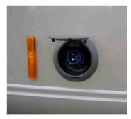
The self-retracting cable reel is behind a separate flap next to the central services unit. Pull out the power cable. Pull again lightly to trigger the selfretracting mecanism.
