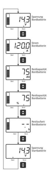
The measuring and display values of the battery computer functions are scrolled forward via button 1 (left)
