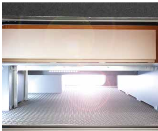
Full-length, heated FRANKIA double floor
