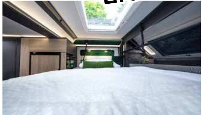
↑ Smart: power drop-down bed that disappears completely into the roof
