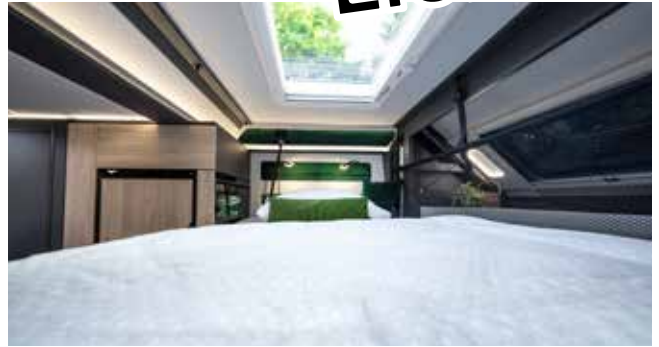
↑ Smart Cruiser: power drop-down bed that disappears completely into the roof (opt.).
