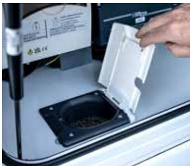
↑ Protected space for the power connection.
