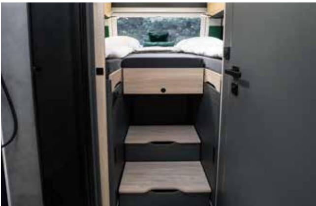
↑ Easier access to the beds thanks to a new step system with rails.
