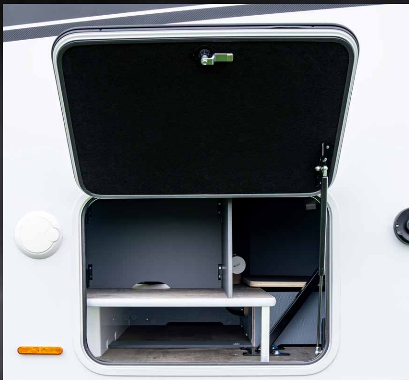
Even more storage space is available beneath the seating area. Smart: accessible from both outside and inside!
